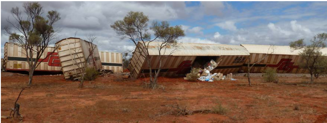
Figure 2: Derailed wagons north side of track.
